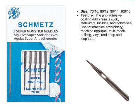
The SCHMETZ Super NonStick sewing machine needle is a Super Universal Needle with a reinforced blade, extra large eye, deep scarf, and a slightly rounded point. The eye corresponds to a needle two sizes larger. If stitching on light or white fabrics or threads, test first for excess residue.
