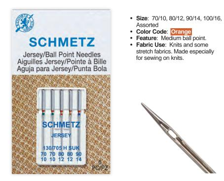
The SCHMETZ Jersey sewing machine needle is also known as a ball point needle. Jersey Needles are recommended when working with jersey fabrics. The medium ball point is designed to avoid breakage of knit fibers at stitch creation.
