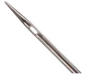
The SCHMETZ Jeans needle is also known as a Denim needle. The advanced point design is a SCHMETZ exclusive. The Jeans needle penetrates thick woven fabrics, denims, and quilts with minimum needle deflection, reduced risk of needle breakage, and fewer skipped stitches. Denim Twin needle available.
