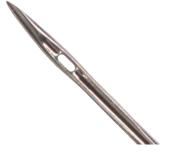
The SCHMETZ Leather sewing machine needle has a left twist cutting point. The cutting point easily penetrates leather. Remember, once the stitch is created, the thread can be removed, but the stitch hole will remain.
