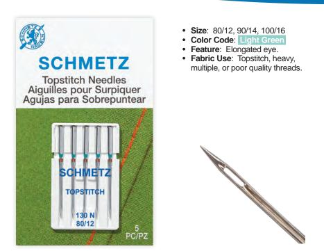
The SCHMETZ Topstitch needle has an elongated eye providing less stress on the thread as it passes through the eye. The Topstitch needle has a slightly rounded point. Achieve perfectly straight and even stitches when using a straight stitch needle plate. A popular needle choice for machine embroidery.
